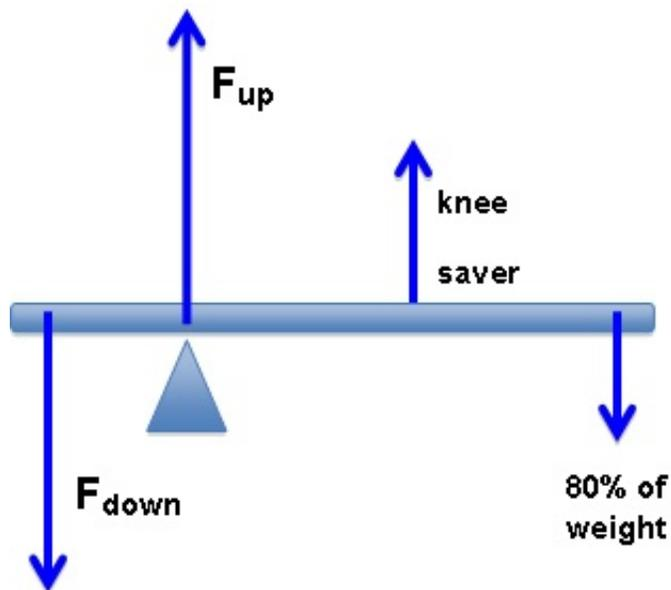
Since we now understand how the forces work in a see-saw, we can add the upward force on the upper body from the Knee Saver as shown above. There are many ways to think about how this additional force reduces the upward force the tibia exerts on the femur, reducing the pressure on the meniscus.
